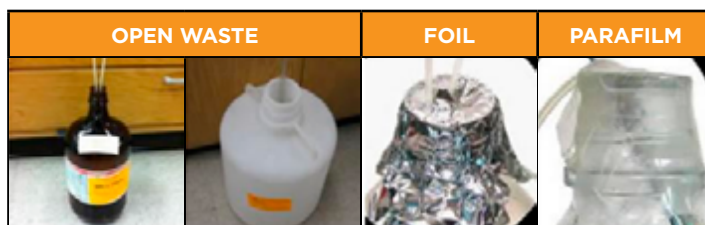
FIGURE 11.5A – Improper LC Waste Collection Processes
