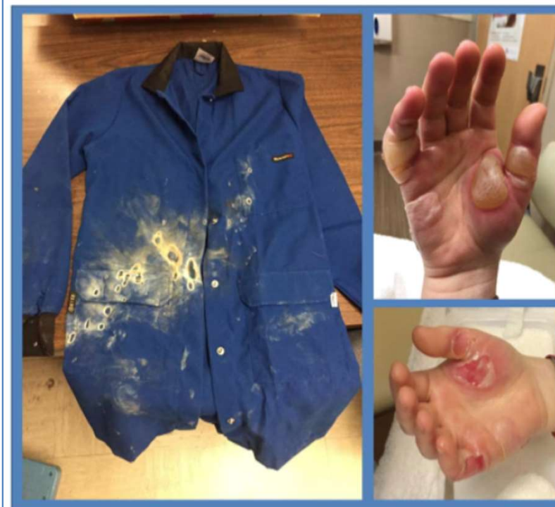
Figure 1.2 A Burn-Scarred Lab Coat Prevented Further Injury to a Chemistry Researcher. A flame-resistant lab coat prevented injury to the researcher's torso during a February 2018 incident involving an air-reactive chemical. However, their gloves did not prevent second-degree burns.
